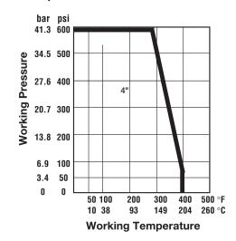
\*See applicable note on reverse side for solder end valves with regards to pressure/ temperature rating.
